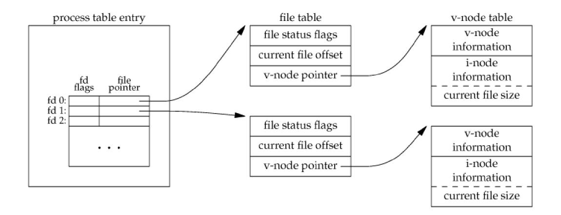
• NOTE: Linux has no v-node, but it has a generic i-node structure. Conceptually, this is same with v-node.
